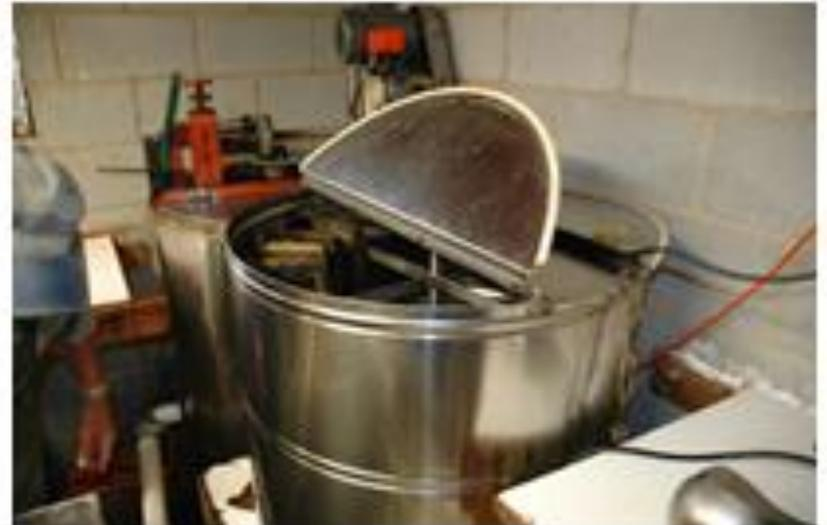
**Mechanical un-capper using an automated hot knife to remove caps.**
